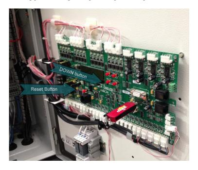
For units that are connected to the internet or to a BMS system the BIN file will need to be updated as well to the corresponding issue number. Using a laptop connect to the Aqua Cooler controller via the Ethernet card in the rear of the controller.
