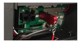
For units that are connected to the internet or to a BMS system the BIN file will need to be updated as well to the corresponding issue number. Using a laptop connect to the Aqua Cooler controller via the Ethernet card in the rear of the controller.
