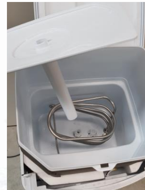
Fig 5 (baffle pipe and shelf)
