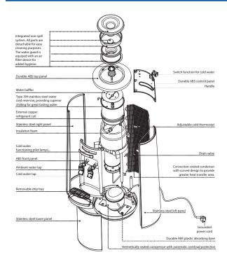
**Note:** Exploded Diagram is of Bottled Cooler
